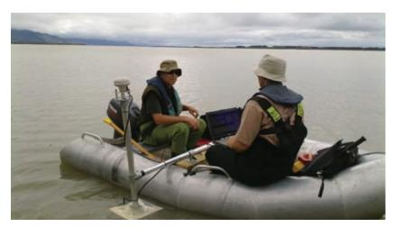
Staff using an echosounder (sonar) during a bathymetric survey in Lake Wairarapa in February. Lake Onoke was also surveyed. A bathymetric survey enables us to measure and map the amount of sediment that has built up over time on the lake bed.
