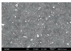
Scanning electron microscopy image of a filter used to collect particulate matter. The larger particles are sea salt. The extremely small particles (white specks) that can just be seen at this magnification are combustion particles that are 50 times smaller than the width of a human hair.
