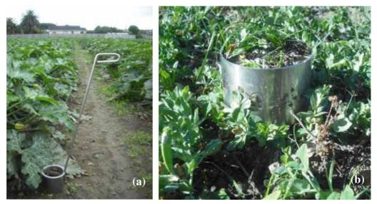
Figure 2.2: (a) Collecting a composite of core samples along a transect using a soil corer. (b) One of three intact core samples taken at each site, to establish the physical properties of the soil.
