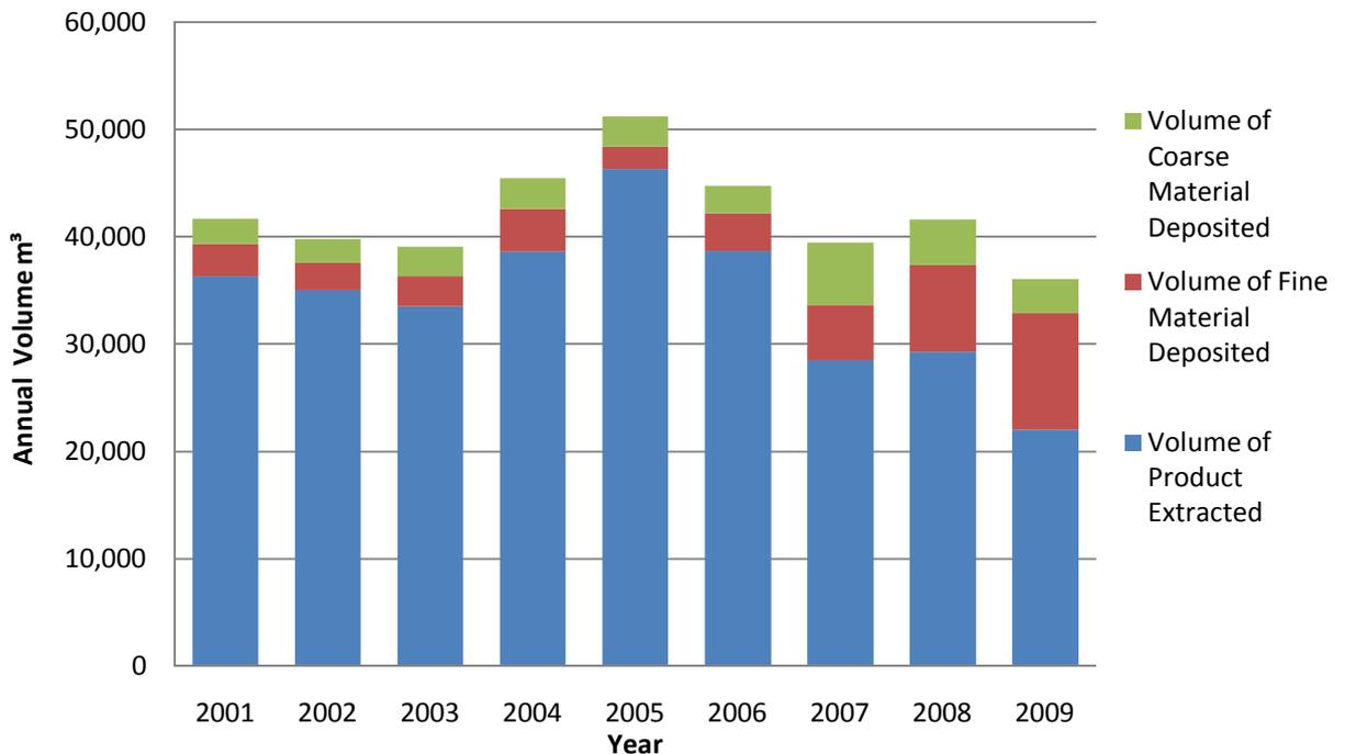
**Figure 12: Annual extraction and deposition volumes 2001–2009; including the volume of both coarse and fine fractions deposited.** Note: Total extraction is the sum of all three volumes each year.
