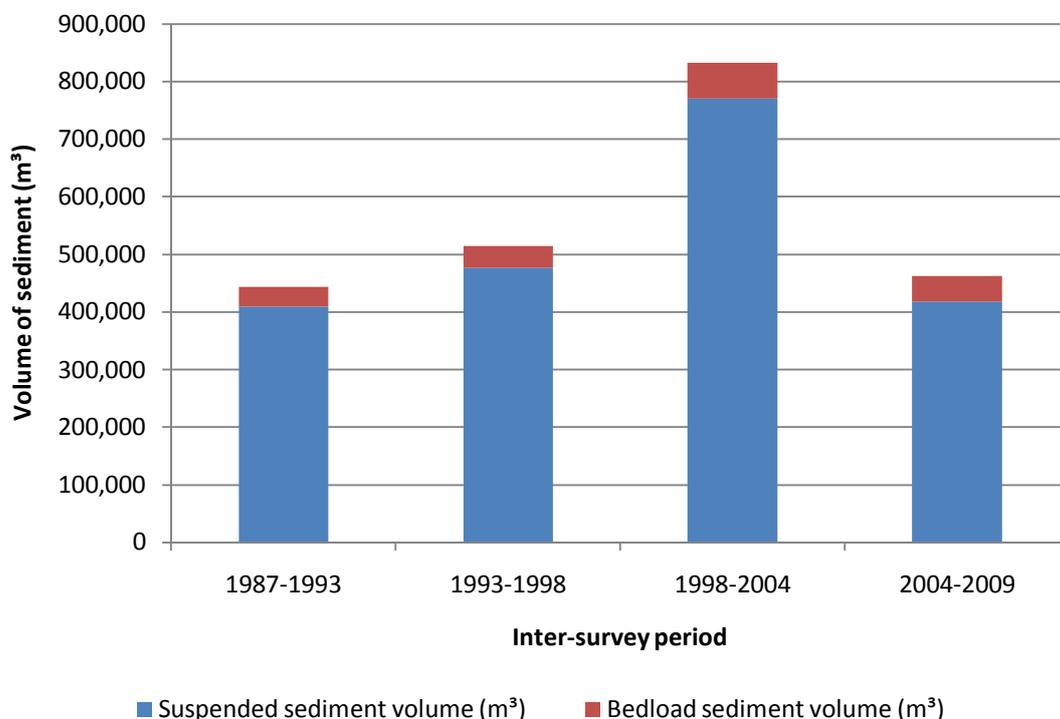
**Figure 7: Suspended load and bedload as a proportions of total sediment transport.**
