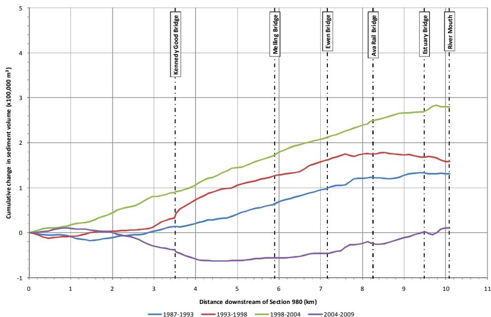
**Figure 8:** Cumulative change in sediment volume in Hutt River downstream of Taita Gorge for each inter-survey period from 1987-2009.
