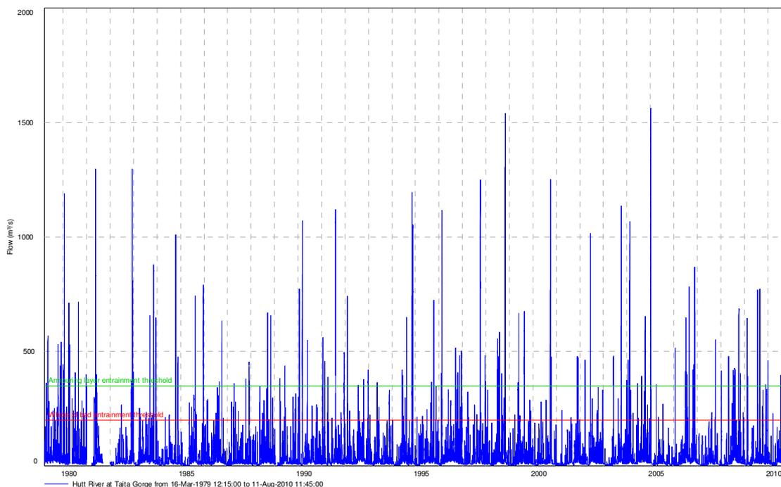
**Figure 5:** Flow record for the Hutt River at Taita Gorge, including two bedload entrainment thresholds (1979-2010).
