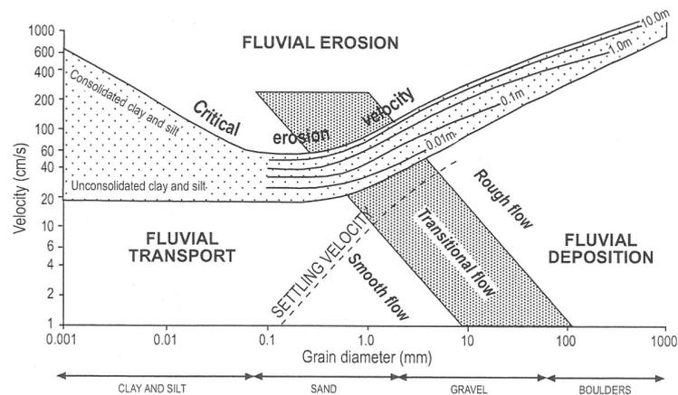
**Figure 2: Erosion, entrainment, and transport thresholds for different size particles (After Sundborg, 1956).**
