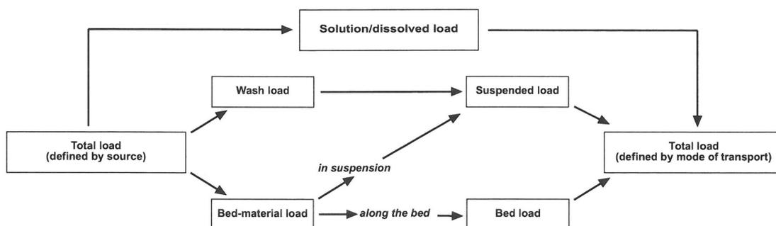
**Figure 1:** The total sediment load of a river can be divided into fractions depending on the primary mode of transport.
