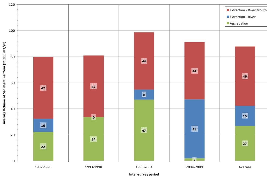
**Figure 9: Average annual sediment deposited downstream of Taita Gorge.**
