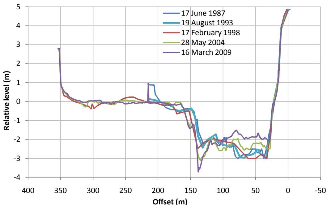
**Figure 15:** Changes in the river mouth cross-section showing general aggradation but deepening of the main channel.
