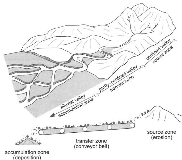
**Figure 3: Characteristic erosion and sediment transport processes down a river profile (Brierley & Fryirs, 2005).**
