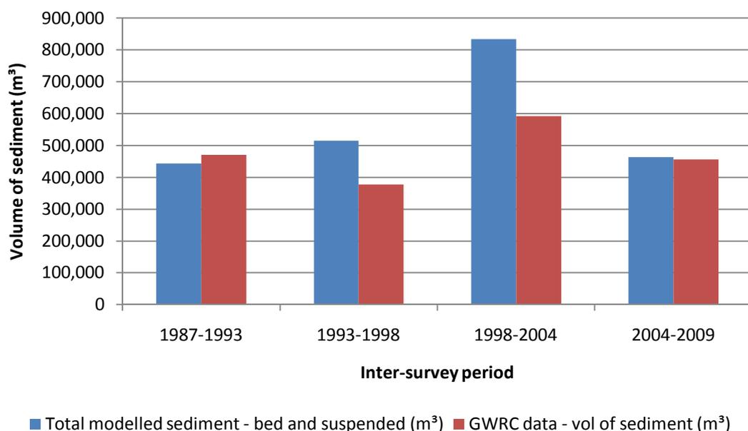
**Figure 6: Comparison of total sediment volumes estimated from modelling and analysis of sediment aggradation and extraction.**
