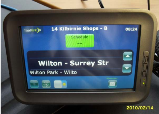
Fig 10.3: On-bus computer and driver display unit
