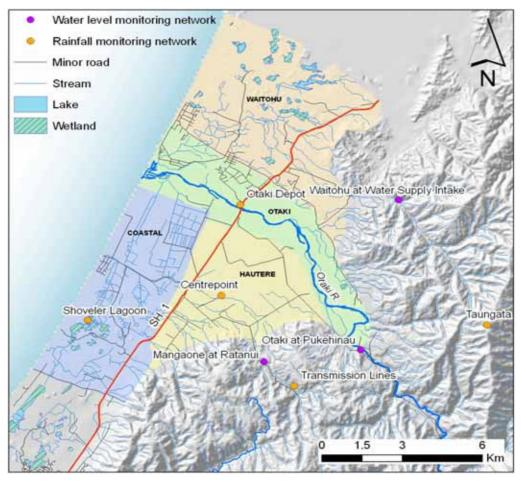
Figure 2.4: Surface water level and rainfall monitoring networks on the Kapiti Coast
