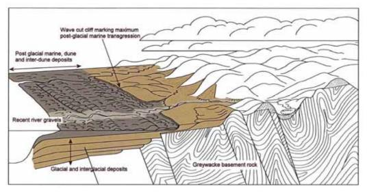
Figure 2.2: General cross-section of the Kapiti Coast geology (Source: Jones & Baker 2005)
