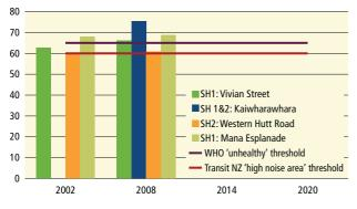
Figure 93: Noise adjacent to arterial routes (noise level 24hr  $\rm L_{eq'}$  dBa, one-week average). Source: GWRC survey, 2008
