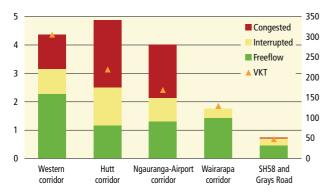
Figure 125: Roading strategic network level of service, 2006. Y-axis: LHS = vehicle hours (000s); RHS = VKT (000s). Source: GWRC Wellington Transport Strategic Model
