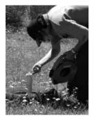
To measure the water depth, lower a weighted tape measure until it touches the water surface. For example, in Figure 6 the groundwater level is calculated as:
