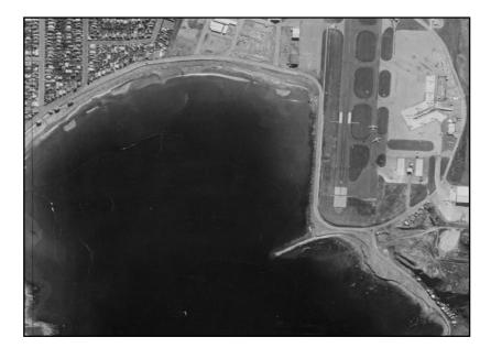
Figure 5a and 5b: Aerial photographs taken in 1945 (top) and in 1962 (below) indicating the significant reclamation undertaken to accommodate the Wellington airport along the eastern end of Lyall Bay (Photograph WCC).
