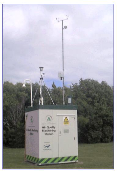
Figure 3.1 Mobile Air Quality Monitoring Station
