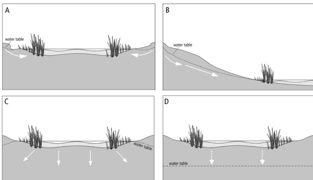
Figure 2: Some wetland/groundwater interactions. The arrows show the direction of flow.
