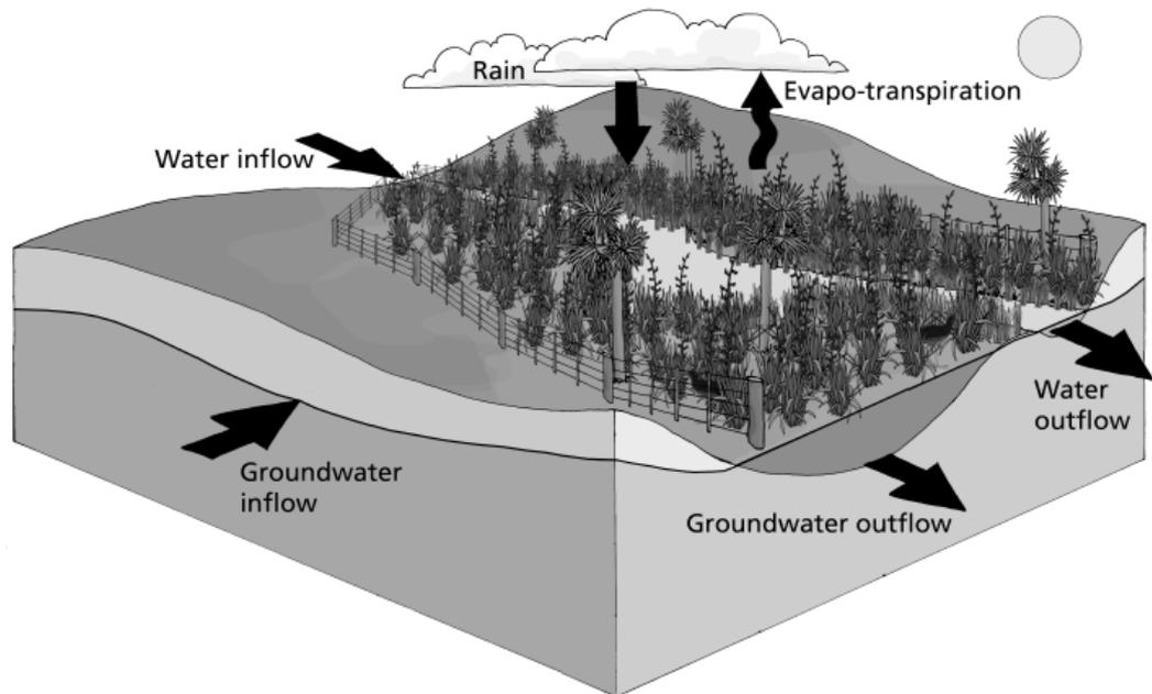
Figure 1: The factors making up a wetland's water balance (after Carter, V, 1996, Wetland hydrology, water quality, and associated functions. In National Water Summary on Wetland Resources. Water-Supply Paper 2425. United States Geological Survey. Washington, DC. <http://water.usgs.gov/nwsum/WSP2425/>)
