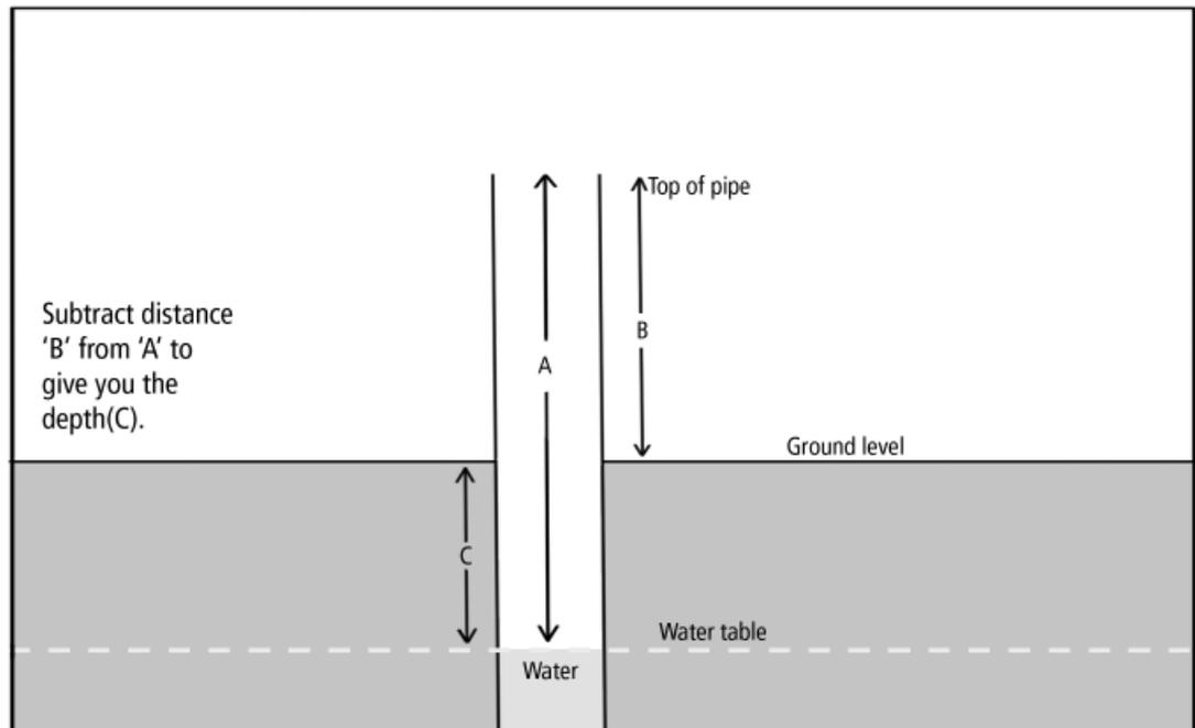
Figure 6: Calculating the underground water level (after Brock, M et al, 2000. *Does Your Wetland Flood and Dry? Water Regime and Wetland Plants*. LWRRDC and UNE, NSW, Australia)
