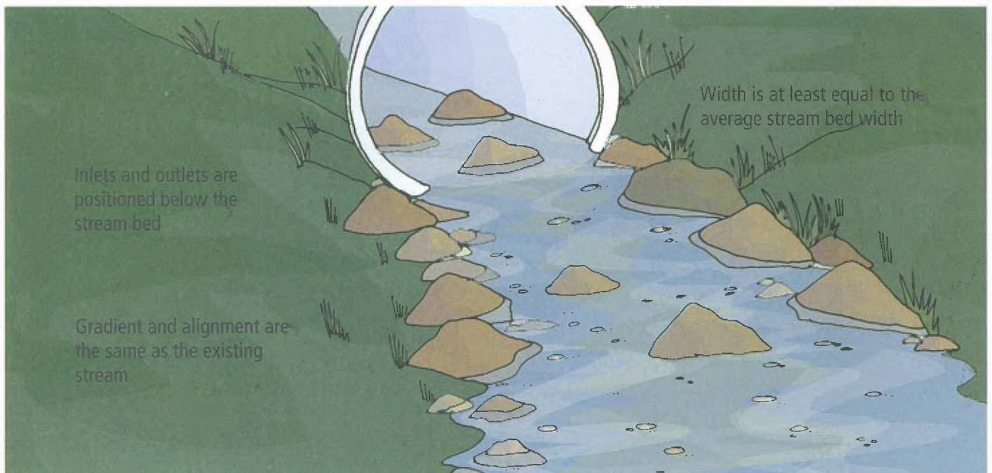
A “low slope” culvert
