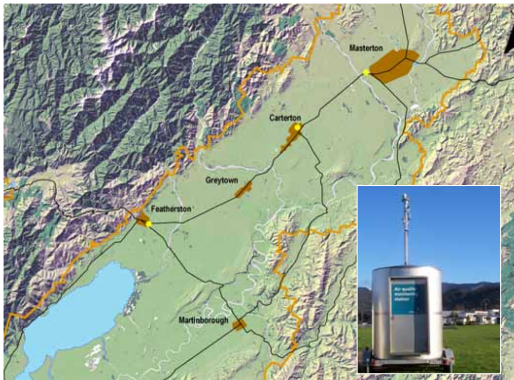
Figure 6.3: Map of the Wairarapa airshed (outlined in orange) showing the location of temporary monitoring sites (yellow dots) in winter 2009. Photo inset shows mobile monitoring station located at Featherston Primary School.
