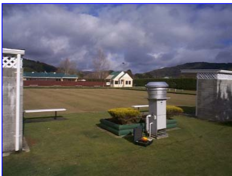
Figure 3.4: High volume sampler at Wainuiomata Bowling Club
