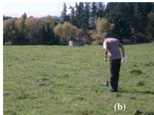
Figure 2.2: (a) One of three intact core samples taken at each site, to establish the physical properties of the soil. (b) Collecting a composite of core samples along a transect using a soil corer.
