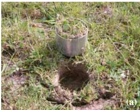
Figure 2.2: (a) One of three intact core samples taken at each site, to establish the physical properties of the soil. (b) Collecting a composite of core samples along a transect using a soil corer.
