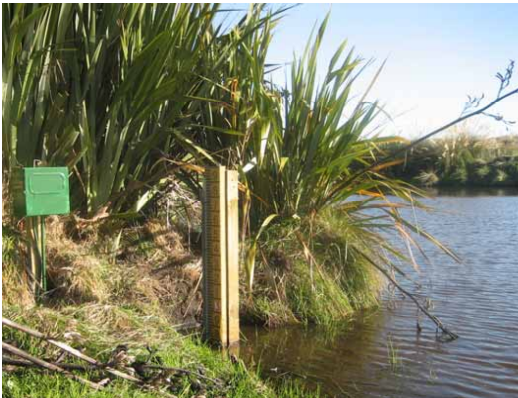
Figure 2.5: Wetland water level gauge installed at Te Hapua wetland on the Kapiti Coast
