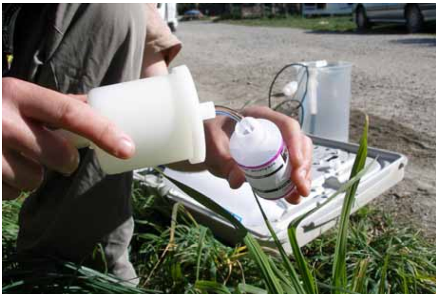
Figure 4.1: Filtering a sample during routine groundwater monitoring
