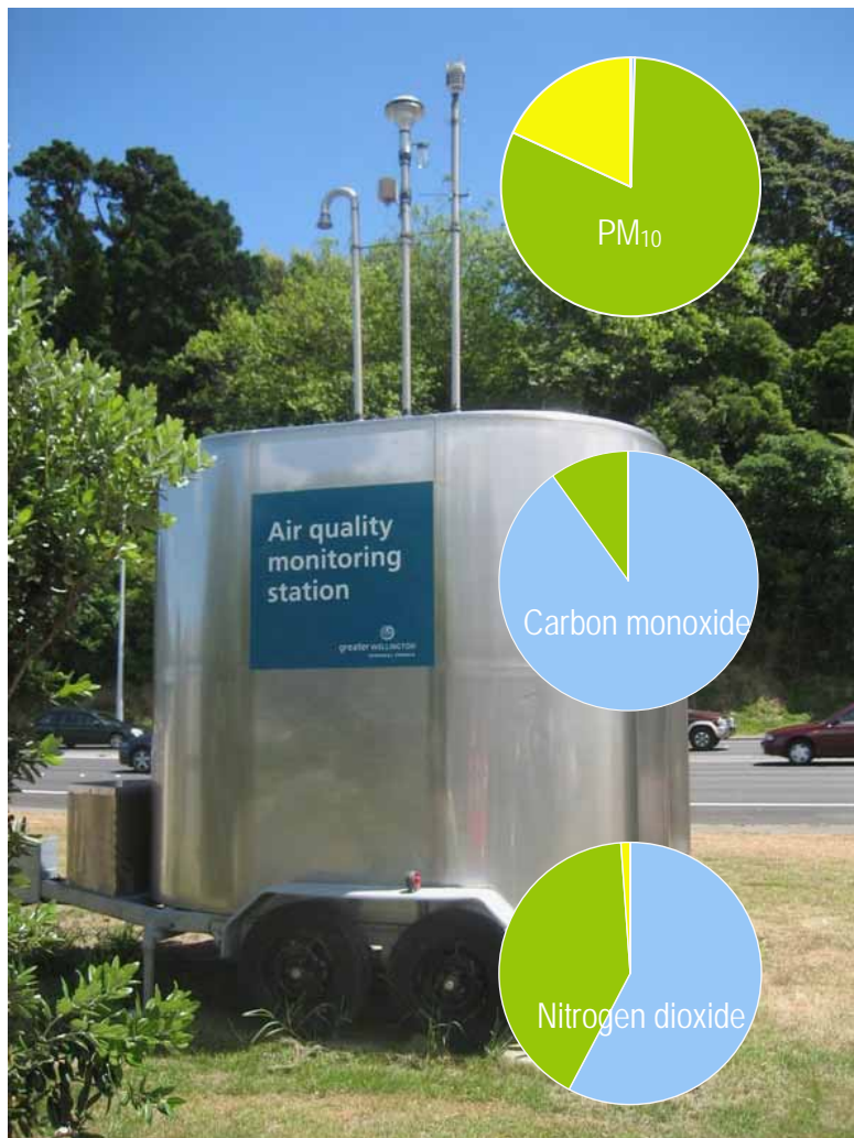
Figure 6.1: Air quality mobile monitoring station at Melling intersection (Lower Hutt) and monitoring results by air quality reporting category for 2008 calendar year
