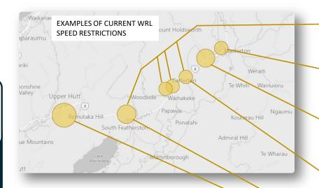
Vibrations (~6min) – Awaiting solution. Speed currently restricted to 60 km/h.
