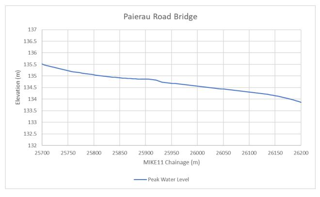
Figure 7-16 - Observed headloss through Paierau Rd Bridge (50 year CC)
