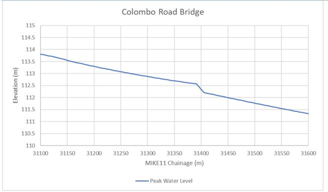
Figure 7-13 – Observed headloss through Colombo Rd Bridge (50 year CC)
