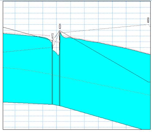
Figure 5-3 – Water level profile at KopuBridges 4221 and 4167
