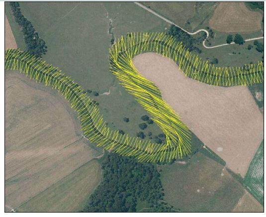
Figure 6-4 - Visualisation of Lateral Link Connections – Taueru River (M11 Chainage 1957 to 3264)
