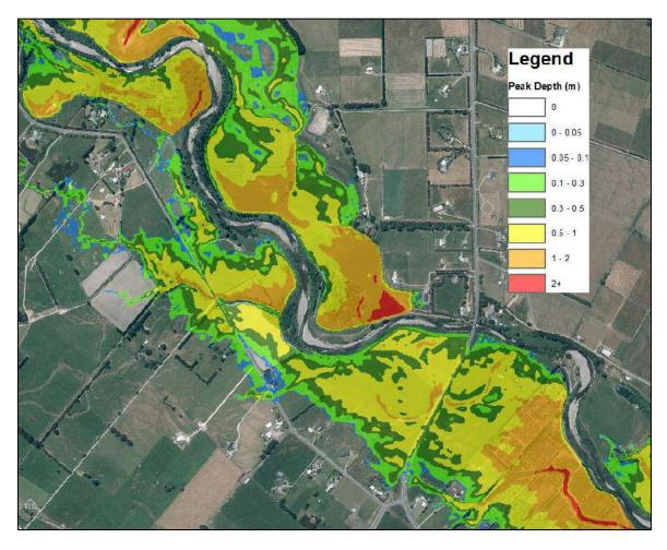
Figure 4-1 – Example of colour scheme used in recent Waihoine River modelling
