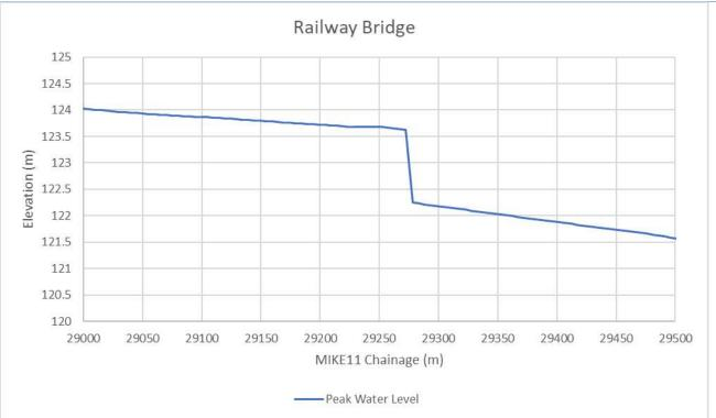
Figure 7-15 - Observed headloss through Railway Bridge (50 year CC)
