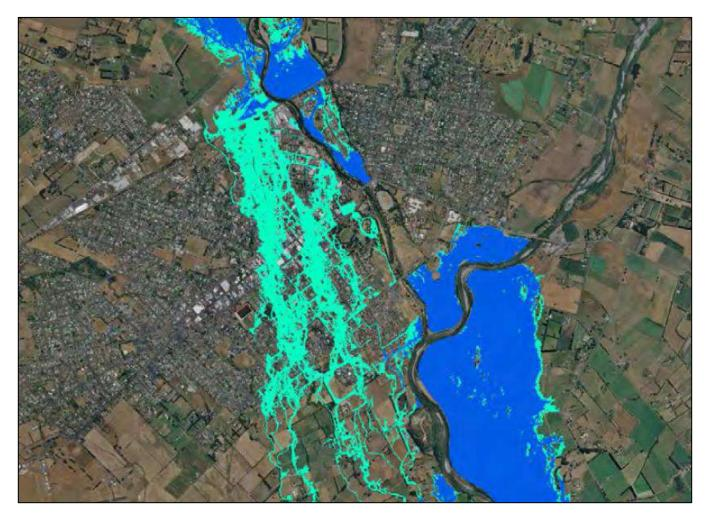
Figure 7-2 - Modelled flood extent showing flood waters overtopping the railway embankment
