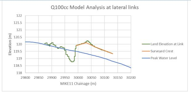
Figure 7-21 – Inspection of modelled links at left bank spill location
