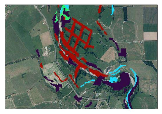
Figure 5-10 - Visualisation of shift due to possible incorrect geographic transformation
