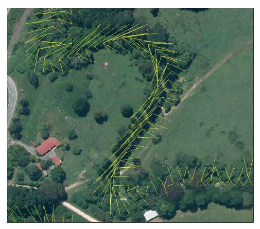
Figure 5-6 – Visualisation of Lateral Link Connections – US\_Kopuaranga MIKE11 Chainage - 4422 - 4945
