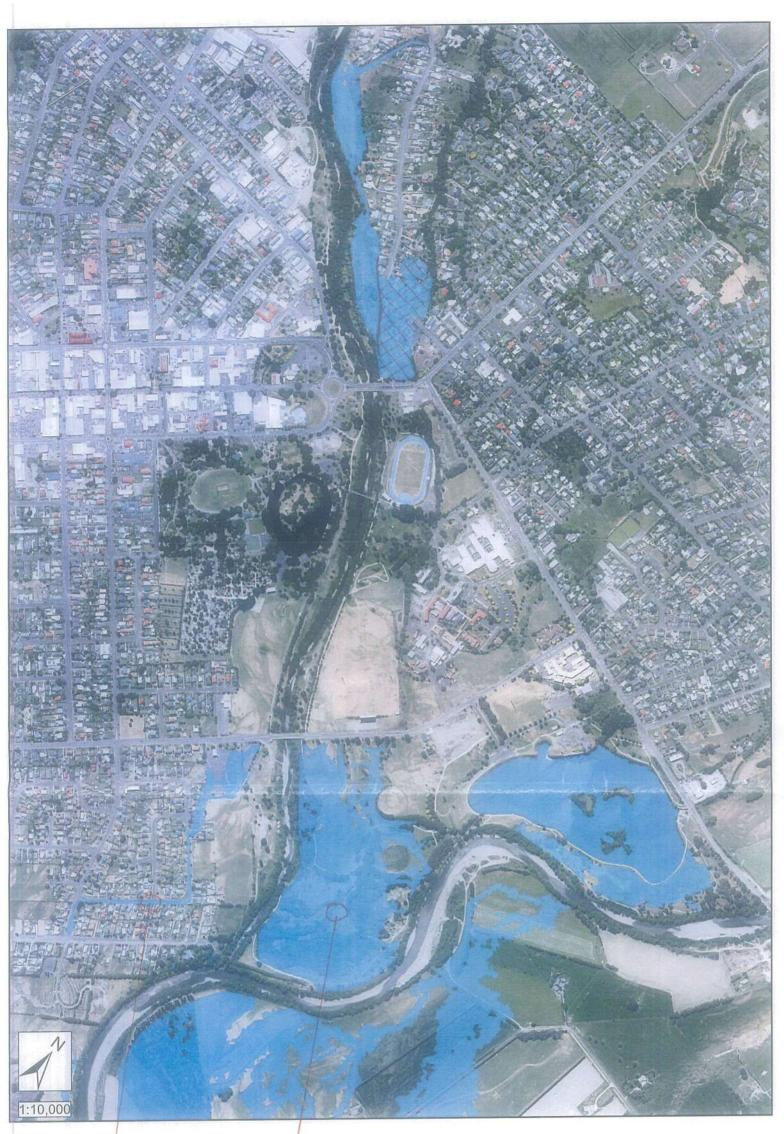
area caused by cut in stop bank during storm water pipe work.
