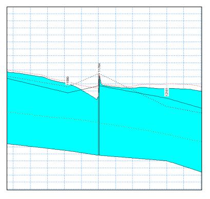
Figure 5-5 - Water level profile at KopuBridge 15583
