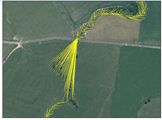
Figure 5-8 - Visualisation of Lateral Link Connections – Whangaehu MIKE11 Chainage 9452
