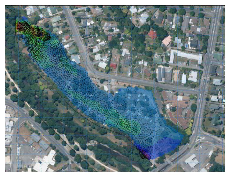
Figure 7-19 - 1998 Calibration results overlaid with vectors showing the direction of flow
