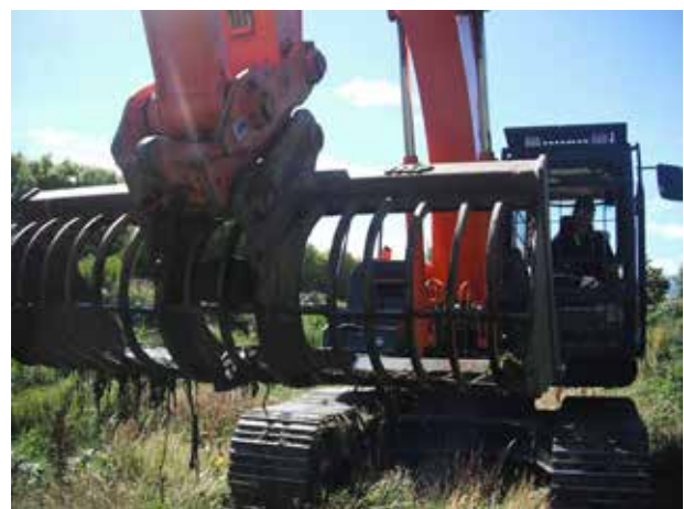
Example of excavators with weed rakes attached. Fish are able to swim through the large gaps and are less likely to be caught than if a standard bucket was used.
